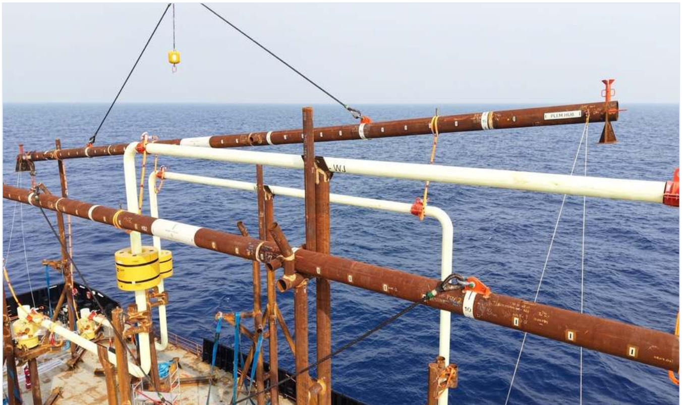
FIG 4.1 — SPREADER BAR PIVOTING ON STERN CRADLE SUPPORT
