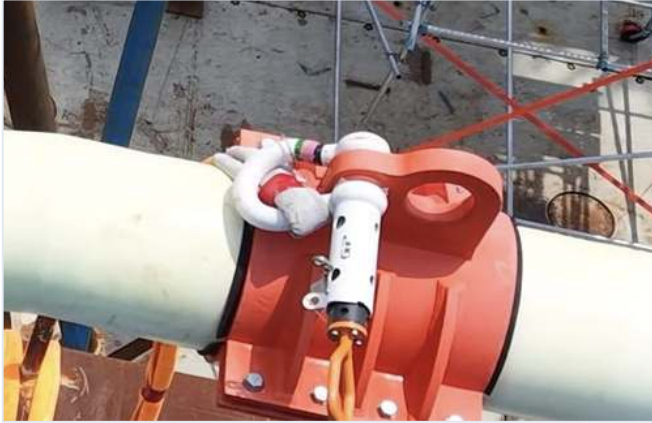
FIG 3.1-A — R-CLIP RETAINED IN ROV SHACKLE, PLEM HUB
